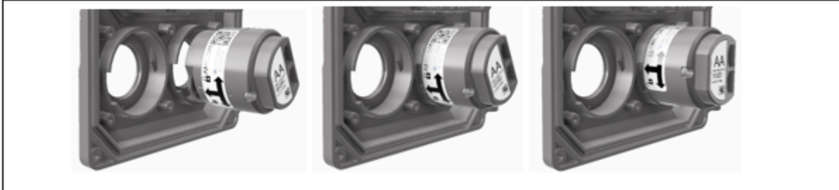
Figure 5-3: Installing Sensor Module
