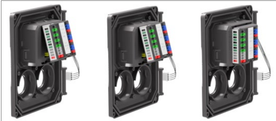
Figure 3-5: Replacing BusPower Module
