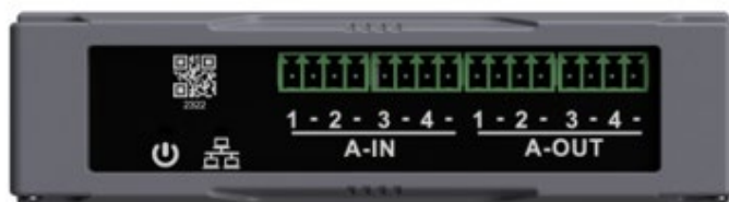
Figure 4-5: CPU Module Analog Input and Output Connections
