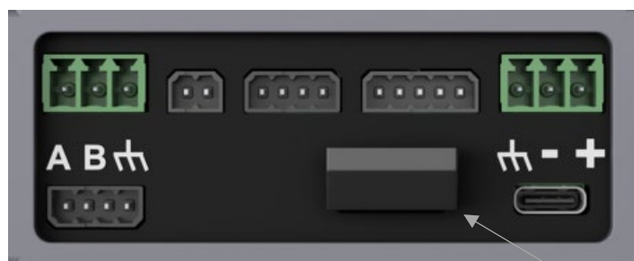
Figure 7-2: RTC Battery Access
