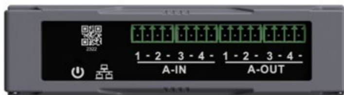
Figure 4-5: CPU Module Analog Input and Output Connections
