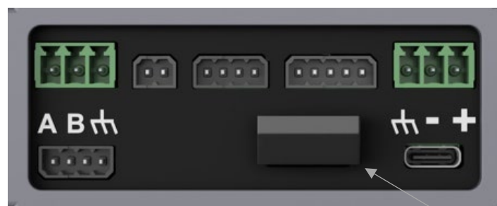
Figure 7-2: RTC Battery Access
