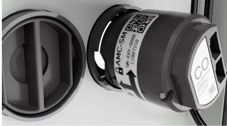
Figure 6-1: Disconnect Sensor Module
