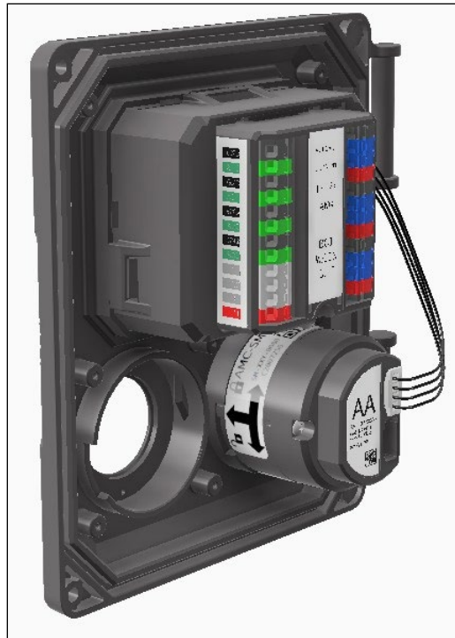
Figure 5-4: Attaching Cable to Sensor Module
