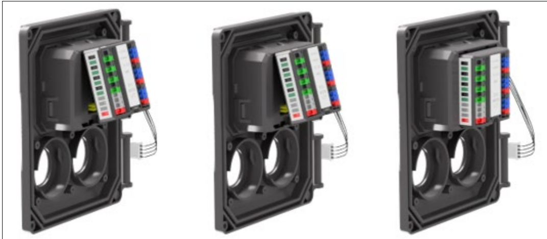
Figure 3-5: Replacing BusPower Module
