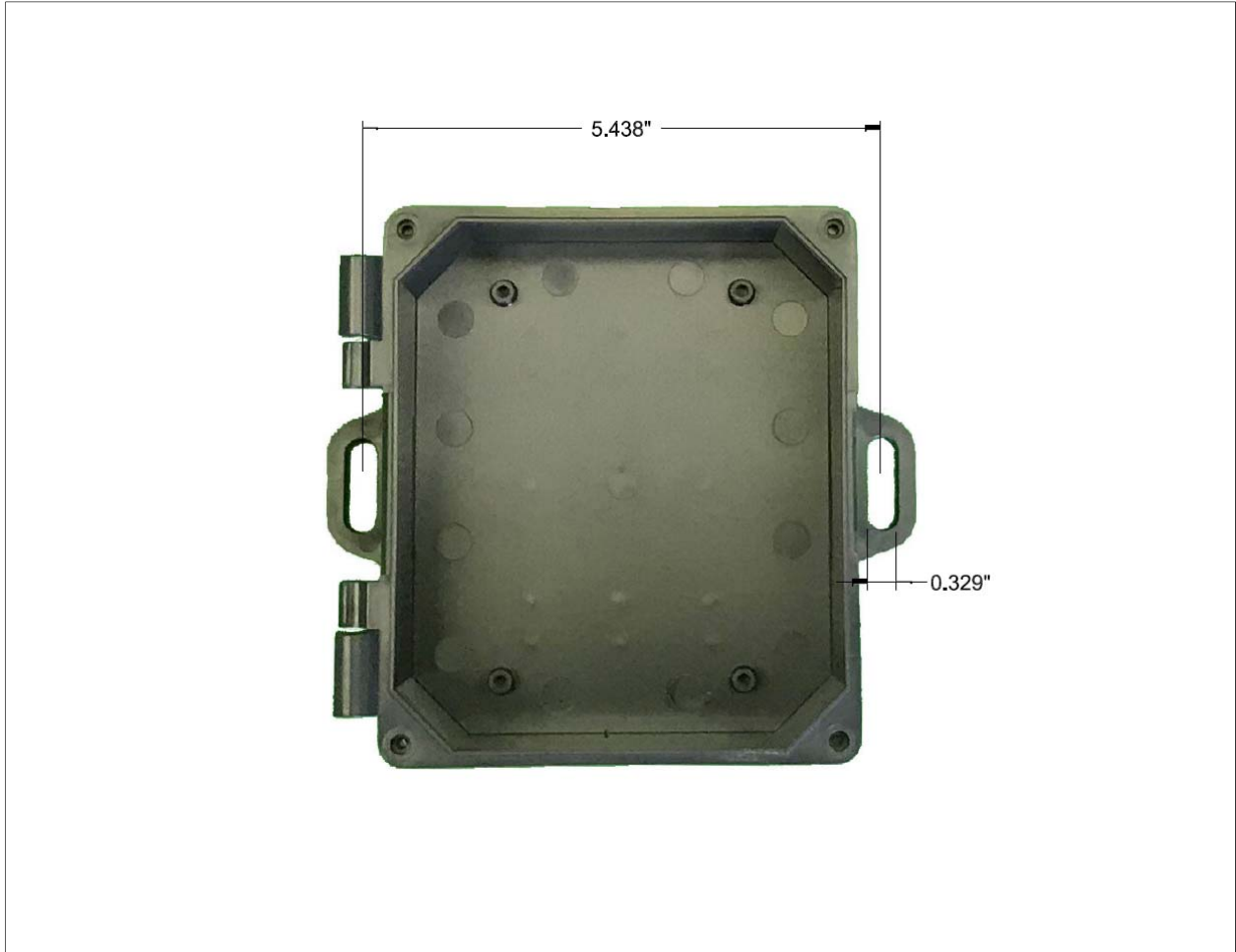
Figure 4-1 Transmitter Mounting Dimensions
